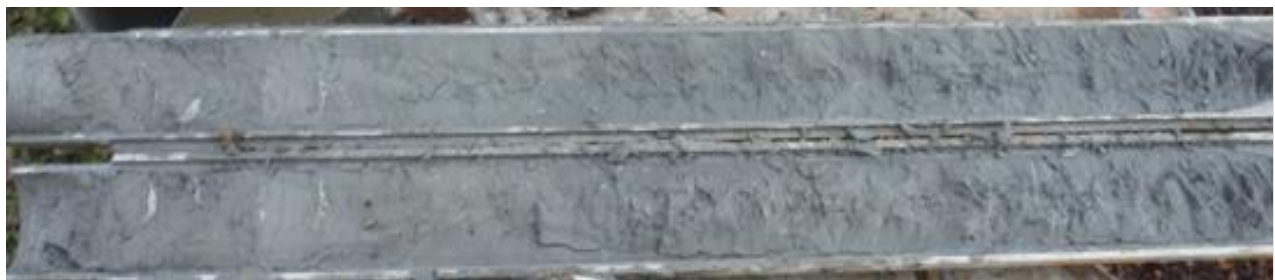
Plate 4. SPT sample of silty, lean clay, showing glacial structures and light gray lenses, PG-1, S-4, 10'.
